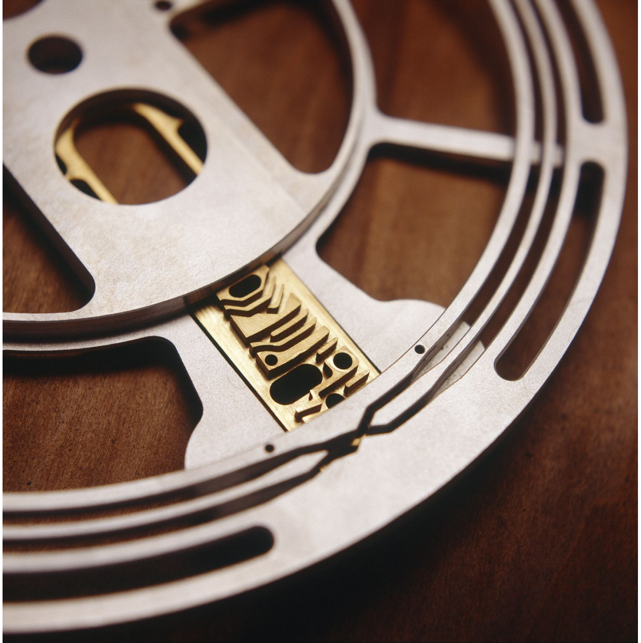
Detail of the clock's adder. Photo: Rolfe Horn, courtesy of The Long Now Foundation.
