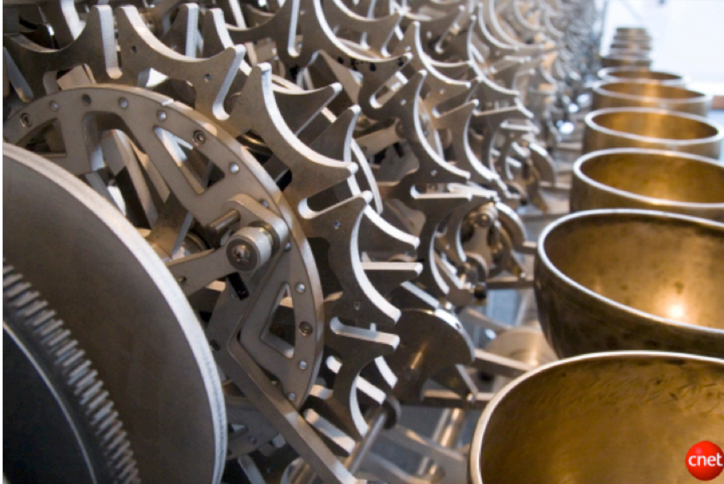
Using a progressive algorithm, large star-shaped plates, called Geneva Wheels, running down the center of the clock will generate a different bell ringing order for each day of the next 10,000 years.
