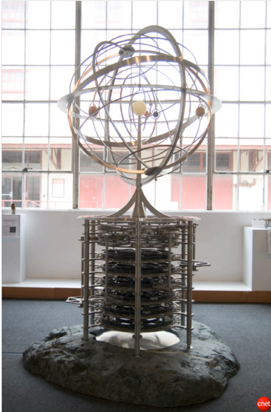
Below the planetary display, each bit serial adder controls one element of the display, the orrery, each of them corresponding to calculate that planet's orbit. The orrery is a spin-off project and the result of brainstorming for the clock, and was completed in 2005.
